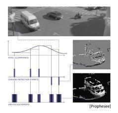
• Neuromorphic computing is particularly effective when implemented on data captured by **neuromorphic sensors**, such as DVS cameras
