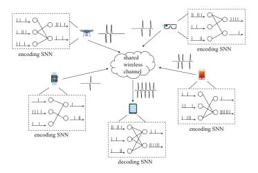
• Neuromorphic communication integrates neuromorphic sensing, impulse radio communications, and neuromorphic computing [Skatchkovsky et al '21] [Chen et al '23]
